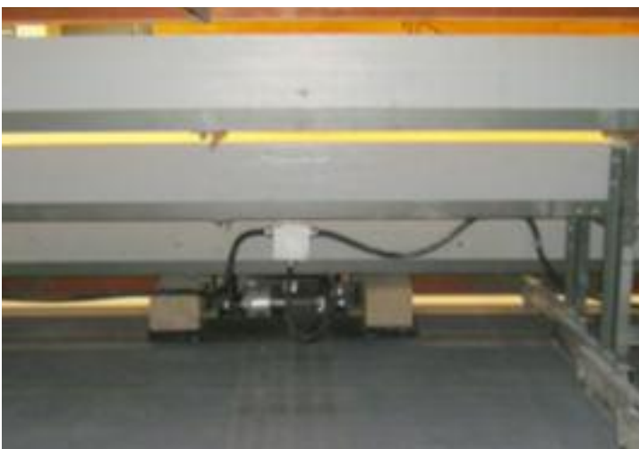
Bleacherman’s heavy duty motorized drive, as seen from the back. Note ballast blocks on either side to add weight and increase traction.
