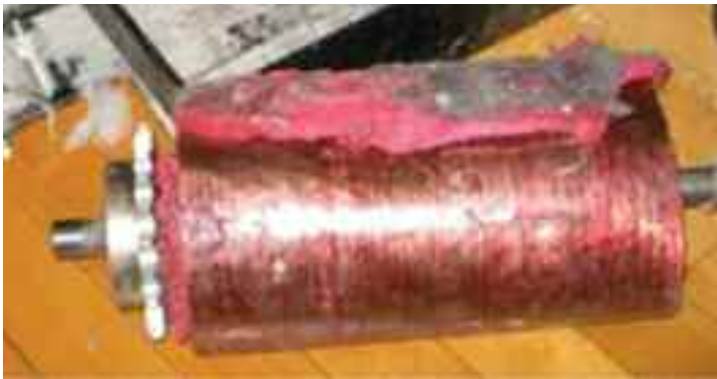
Typical drive roller showing deterioration and delamination of the outer covering from the metal roller. We replaced five existing motors with our heavy duty motors equipped with 50-durometer drive rollers that won't delaminate, guaranteed.
