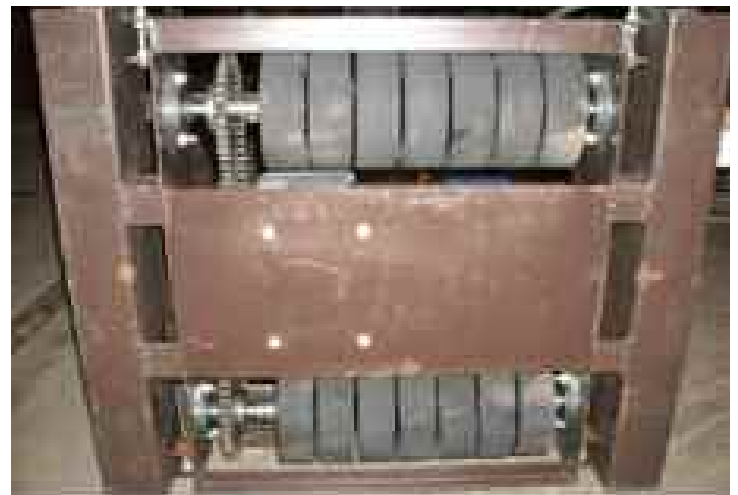
Bottom view of Bleacherman's heavy duty motor drive replacement shows two rows of 14-inch wide drive wheels for maximum traction.
