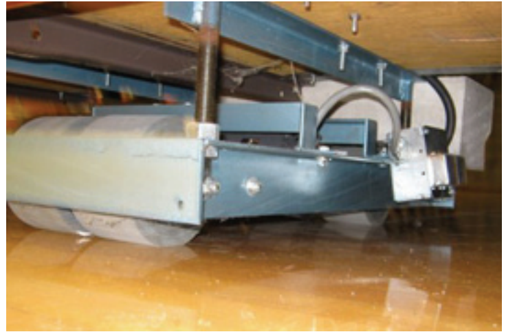
Motor drive seen from front, has no counter weight to offset the 90-lb weight on the back.
