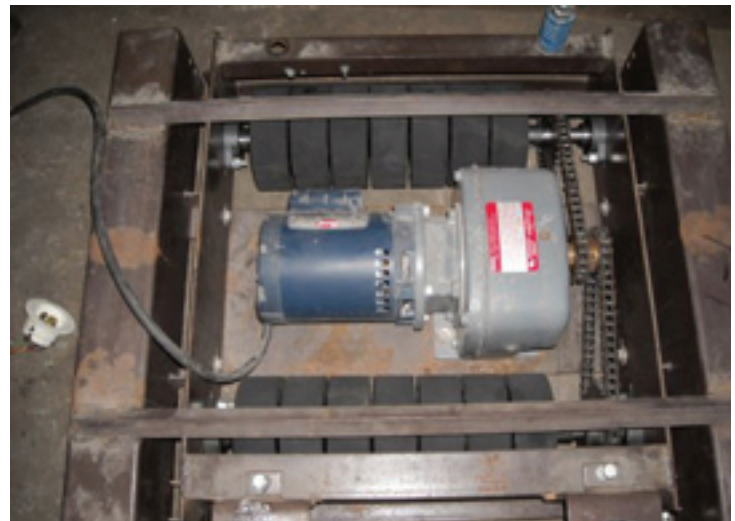
Top view of drive system with Bleacherman drive rollers. All useable components such as frame, motor, gear drive, are reused.
