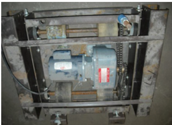
Top view of drive unit with original 4-inch drive rollers.
