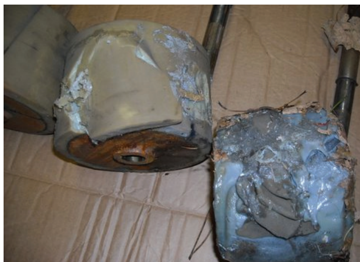
The synthetic covering on these drive rollers are breaking down, and peeling away from the steel drive roller core.
