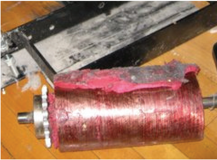
Here the delaminated drive roller has been removed from the motor drive frame
