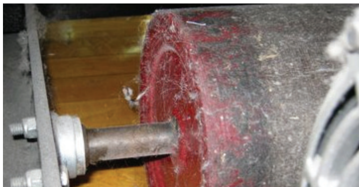
Delaminated drive roller. The urethane covering has peeled off, leaving a bare steel cylinder. This will damage the floor, whether wood or synthetic. ($$$$)
