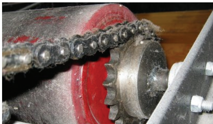
Another view of a completely delaminated drive roller. .
