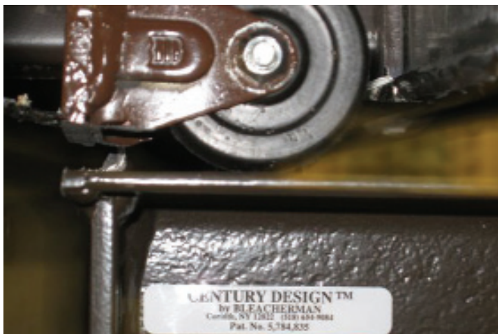
A close-up of the Century Design® wheel on the runner in the full open position.
