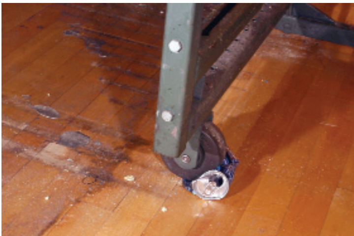
Keeping the area beneath the understructure clean and free from debris is required. Obstructions can prevent the wheels from turning freely and cause damage to the floor.
