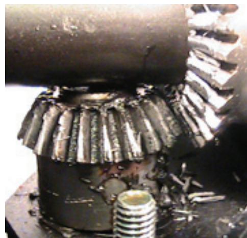
Close up of damaged teeth on beveled gears. Gears and motors were damaged due to sagging and had to be replaced.
