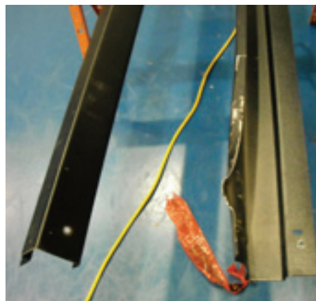
Comparison of new replacement nosebeam and old damaged nosebeam.
