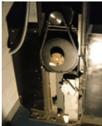
Motors for reverse-fold, non-friction drive are located underneath the platforms. It's dark back here!
