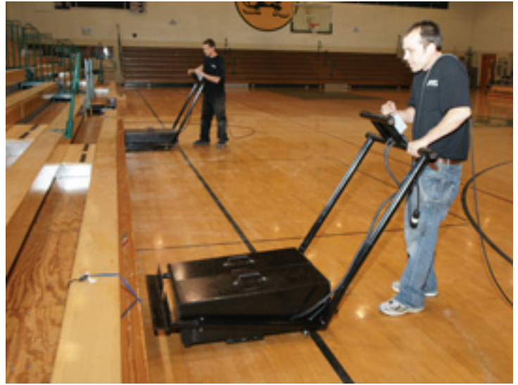
All five banks of telescopic bleachers are opened and closed with a two-man "mule team." Mule can be converted to a motorized drive mounted below the bleachers at a later date.
